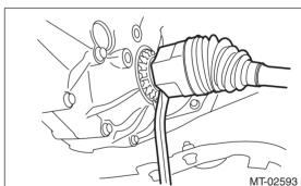
10) Remove the differential side retainer oil seal.
