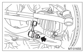
8) Remove the bolt securing the ball joint of the front arm to the housing, then separate the front arms and the housing.
